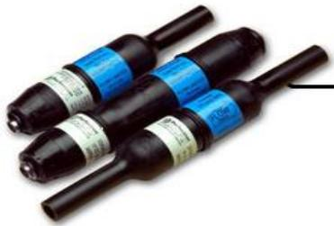
An Excess Flow Valve (EFV) is a mechanical device installed inside a natural gas distribution service line between the street and meter. EFV's are designed to shut off the flow of natural gas automatically if the service line breaks. EFVs are designed so that general usage, such as turning on appliances, will not trip the valve.
